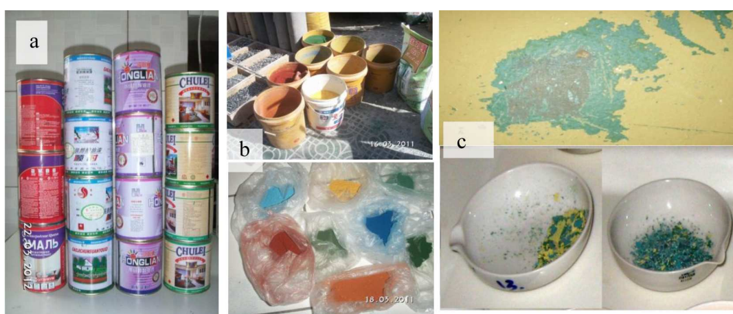
Figure 1. The selected samples of oil paints (a), ochre paints (b), and scraped from wall of the NUM oil paints (c)
